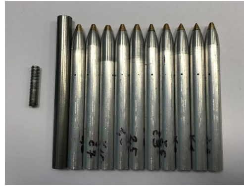
Figure 1. Pitot tube wind tunnel installation (left) and ten pitot tubes with various inlet diameters (right)
