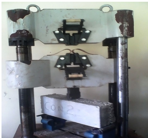
Fig. 2. Beam under load
