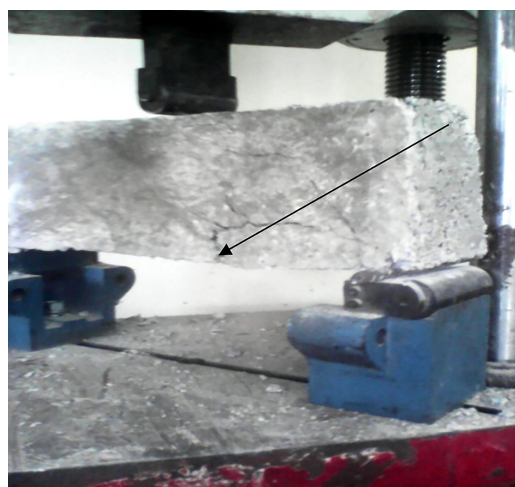
Fig. 9. Bending moment cracks in beam with polypropylene grains
