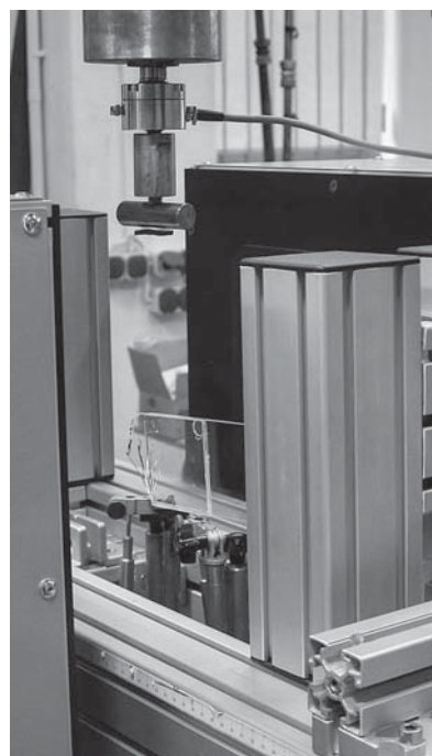
Fig. 8. Glass specimen in StrainMatic measuring machine (photo by T. Serafinavičius)
