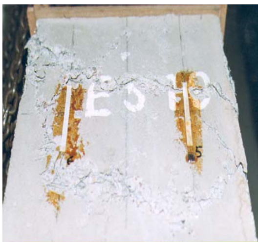
Fig 10. Character of destruction of column with fibre concrete head, made of the same concrete mix as the whole column (S10-F)
