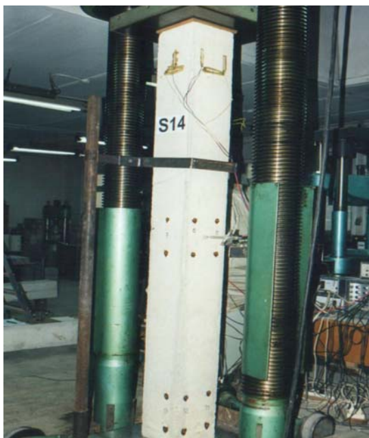
Fig 1. Testing stand of the columns
