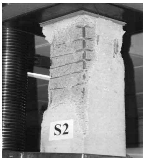
Fig 4. Character of destruction of composite columns loaded over the composite cross-section
