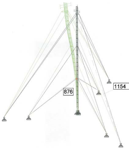
Fig 2. Mast displacements when the guy 1154 does not operate
