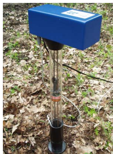
Fig 2. Surface magnetic workability measuring sensor
