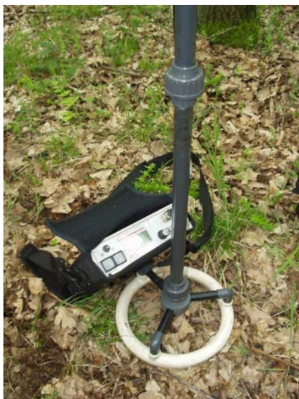
Fig 3. Vertical magnetic workability sensor
