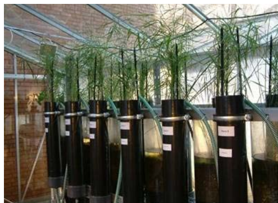
Fig 4. Leaching column experiment for investigating the mobilisation and plant uptake of metals by application of EDTA to soil
