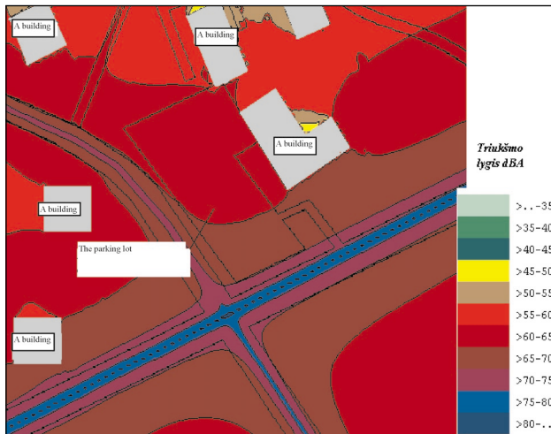
Fig 8. Results of the simulation of noise dispersion at the parking lot on Ateities street
