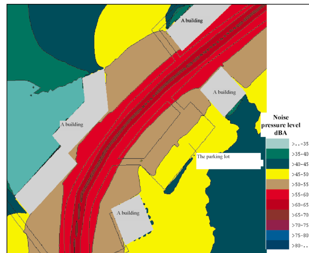
Fig 7. Results of the simulation of noise dispersion at the parking lot on Architektų street
