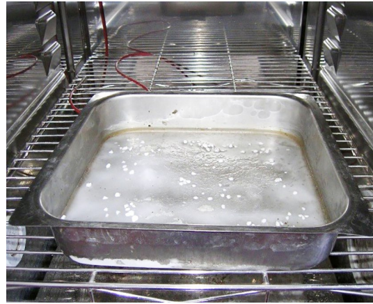
Fig. 3. Formed ice sample with an applied DM
