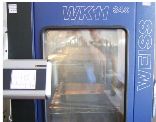
Fig. 4. Climatic chamber, where the sample was kept at different temperatures
