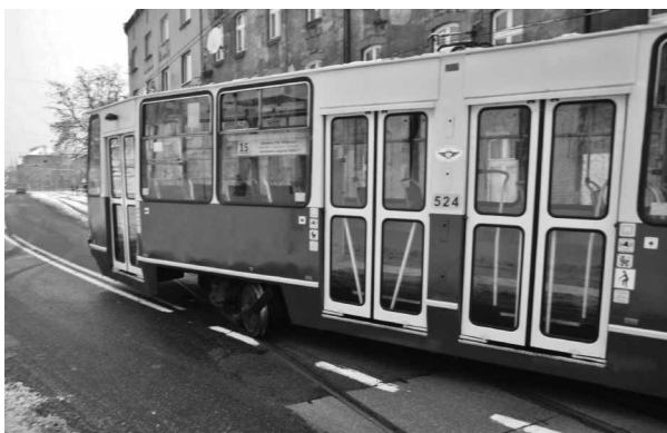
Fig. 8. Tram derailment over a switch
