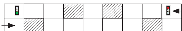
Fig. 3. Traffic regulation for the travel through a chain of road construction works sites in a mode of the unidirectional “green wave”
